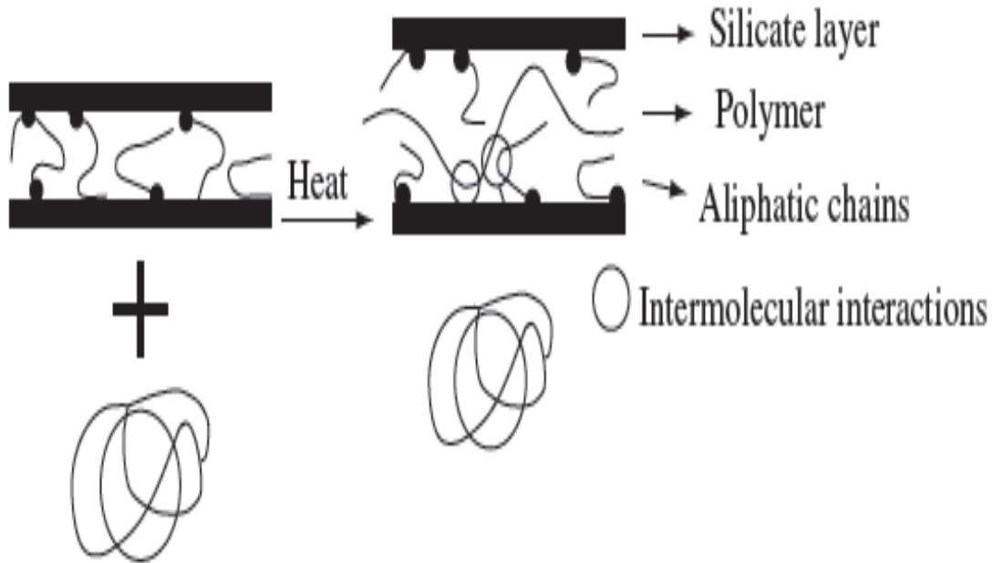
**Figure 1: Melt intercalation synthesis of polymer/clay nanocomposites [1]**
