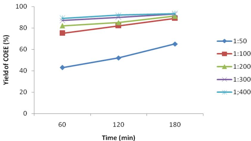
Fig.3. Influence of oil to alcohol molar ratio during reactive extraction of Castor seed; Other parameters: Catalyst concentration = 1%, temperature = 75 °C, mixing speed = 600 rpm
