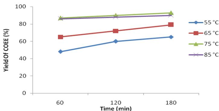
Fig.4. Effect of temperature during reactive extraction of Castor seed: Other parameters: alcohol to oil molar ratio= 300:1, catalyst concentration = 1%, mixing speed = 600 rpm
