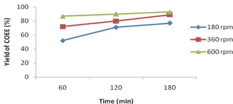
Fig.5. Effect of agitation speed during reactive extraction of Castor seed
